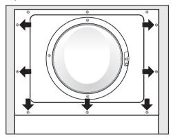
■ Screw the front panel to the machine door.
